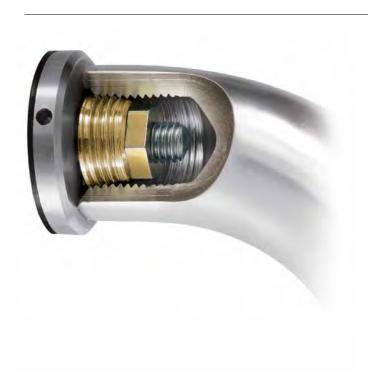
FSB's clamping-rose fixing method enables pulls to be tightened fast against the surface of the door. The visible fixing screws otherwise required are done away with.
